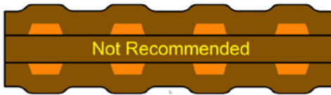
Figure 4.7 Adjacent-layer copper traces are not recommended
