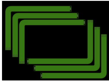
Figure 5.10 Embedded Board Array panelization of the CNC gantry flex circuit
